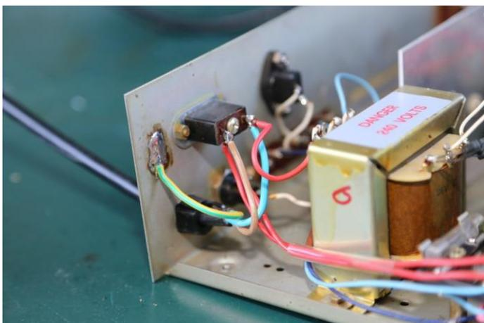
Recently, a colleague from church dropped off this ancient Diamond brand amplifier that he picked up at the tip shop? All it needed was a new power cord. I'm not sure how the original cord was anchored, as all that was left was half a rubber grommet, no clamp etc.
