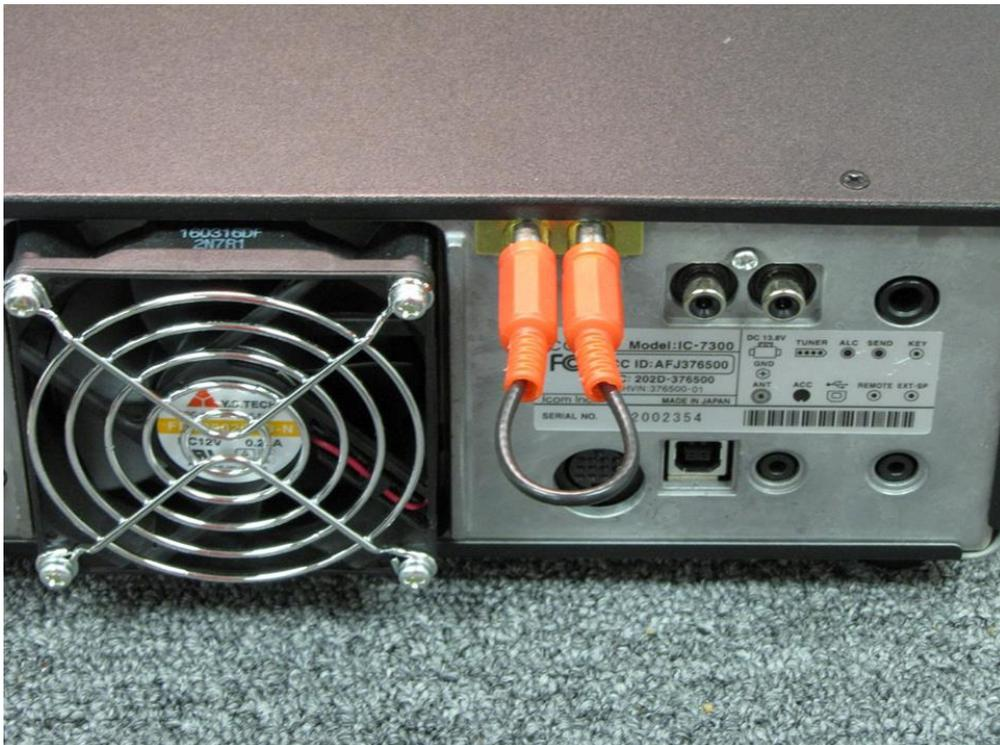
The INRAD model **RX7300** allows the user to add a receive-only antenna jack to the Icom IC-7300. This easy to install plug-in modification requires no soldering and is simple to install and easily reversible. The RX7300 can also be used for the insertion of accessory items into the receiver chain on the IC-7300 like receive-only bandpass filters, low noise preamps, etc.
