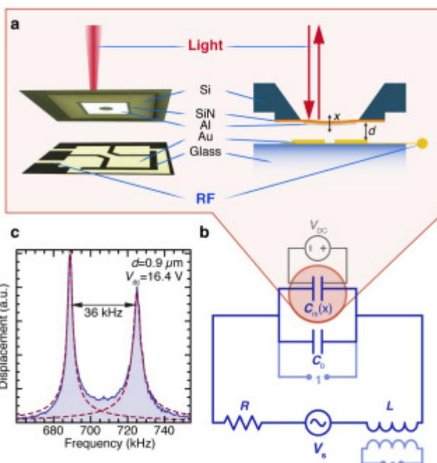
The trick that Bağcı and co have pulled off is to bounce a laser beam off the nanomembrane causing an optical phase shift that they then measure using standard optical techniques.
