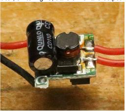
I connected the earth clip of my scope test lead to the probe tip (making a pick up coil) and looped it around the assembled light. and I soon had a semi-stable signal on the scope screen. So yes, they do radiate.
