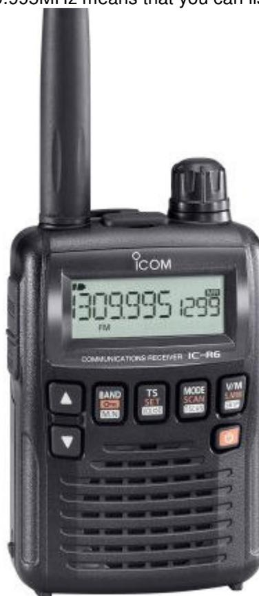
easy, thanks to the IC-R6's ability to operate from a variety of power sources. The standard BC-07 AC adapter or optional cigarette lighter cable, CP-18A/E allow for simultaneous battery charging while operating the radio, a useful function while using the IC-R6 in your vehicle or at home. The receiver can also be powered by the optional BC-194 charger stand which eliminates the need to connect and disconnect an AC adapter to the DC power jack of the receiver.
