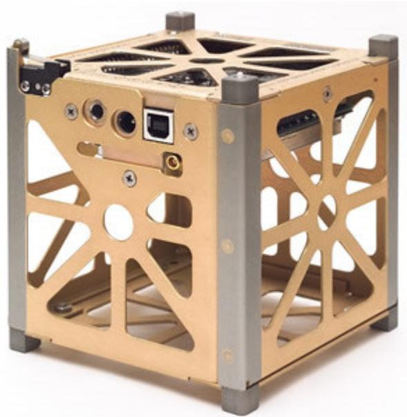
Montana State designated its satellite as Explorer 1 Prime, or E1P. The name honors the launch and scientific discoveries of the Explorer-1 mission, which detected the Van Allen radiation belts more than 50 years ago. E1P will carry a miniature Geiger tube to measure the intensity and variability of the electrons in the Van Allen belts.
